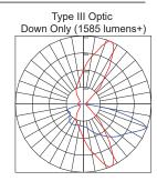
\*Based on 12L down only +12 watt, Lumen output of type III optic varies from standard COB modules - see Tessera 3101 specification sheet for details.
